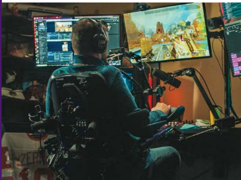
The Augmental MouthPad^ uses a mouth device for both head and tongue control.
