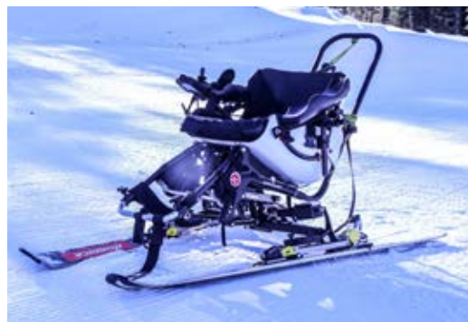
The TetraSki uses advanced Bluetooth sip-and-puff technology that could be used in other devices.
