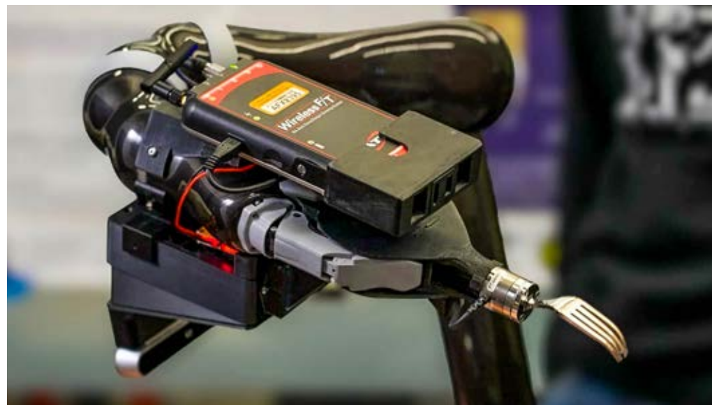
The Assistive Dexterous Arm is controlled through an app to help people feed themselves.
